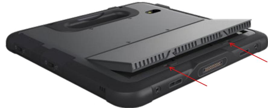
To swap the battery, lay the tablet on a flat surface, and pull the two tabs indicated towards the edges of the tablet. The battery will pop loose and a replacement can be slid into place.
